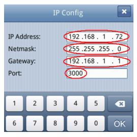
Figure 6-7 Set the network parameters of the oscilloscope
