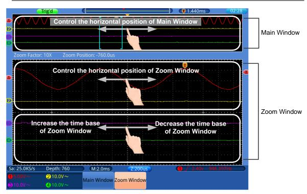
When **Main Window** in the bottom menu is selected, the horizontal operations using touchscreen are shown in the figure below:
