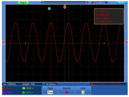
Figure 5-11 Waveform of Time Cursor Measurement
