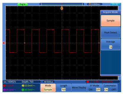
Figure 5-3 Normal ACQU Mode display, in which no burr can be detected.
