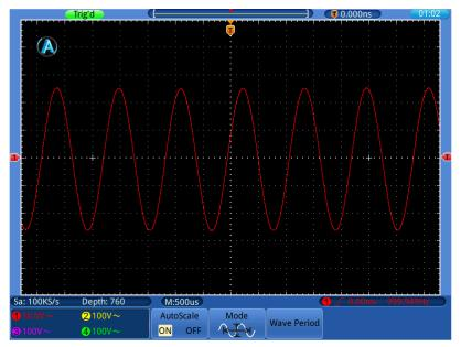
Figure 5-14 Autoscale Horizontal-Vertical multi-period waveforms
