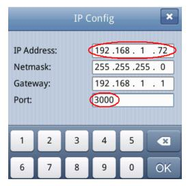
Figure 6-4 Set the network parameters of the oscilloscope
