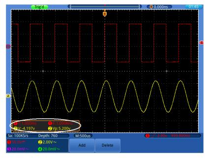
Figure 5-7 automatic measurement
