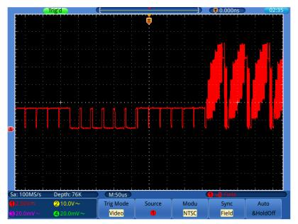
Figure 7-7 Waveform Captured from Video Field Trigger
