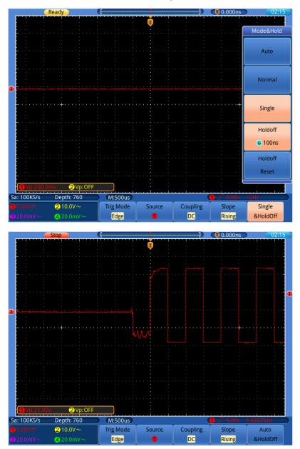
Figure 7-3 Capturing a Single Signal
