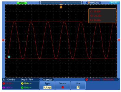
Figure 5-10 Waveform of Voltage Cursor Measurement
