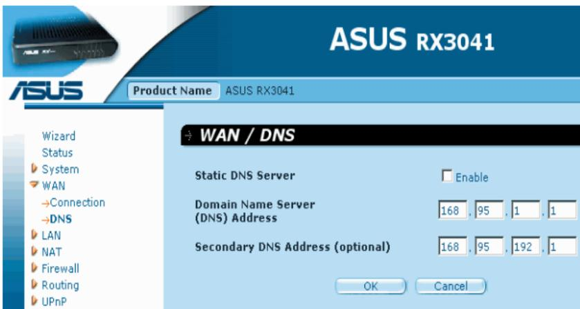
**Domain Name Server (DNS) Address:** This is the IP address of the DNS server provided by the ISP; or you can specify your own preferred DNS server IP address.
