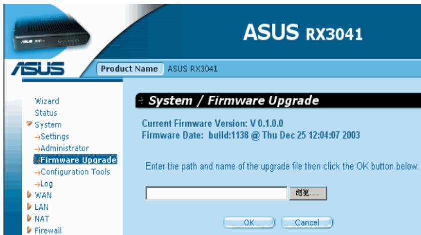
**Firmware Upgrade:** This tool allows you to upgrade the router's system firmware. To upgrade the firmware of your router, you need to download the firmware file to your local hard disk, use the Browse button to find the firmware file on your PC.
