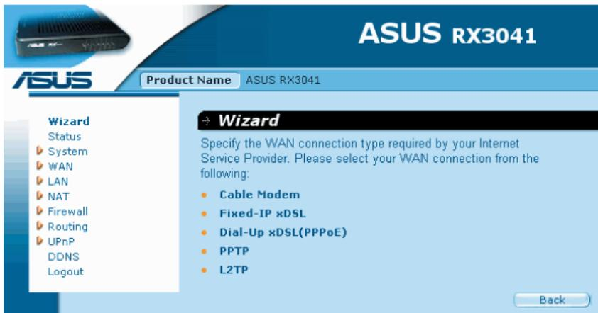
**Cable Modem:** If your router connects to the cable modem, click Cable Modem to enable/disable the MAC cloning function (MAC address is provided by your ISP).
