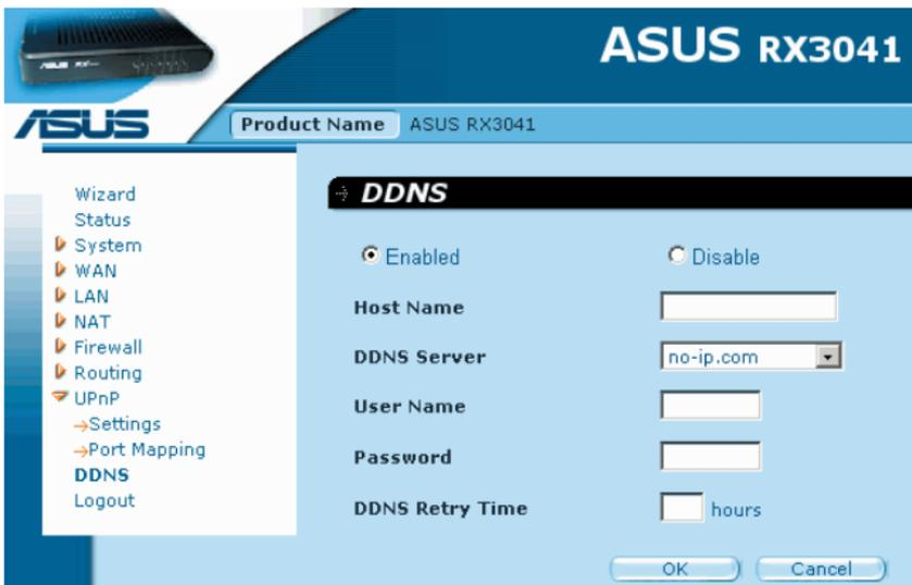
**DDNS:** Enable/Disable the DDNS function of this router.
