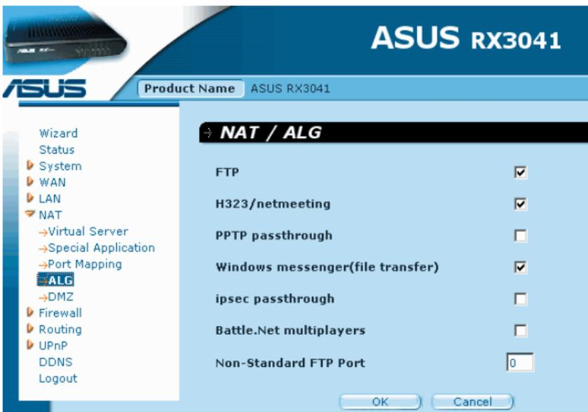
**ALG (Application Layer Gateway):** You can choose to enable ALG, then the router will let that application correctly pass through the NAT gateway.
